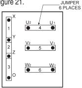
Figure 21. Voltage Change-Over Board 240V Configuration
